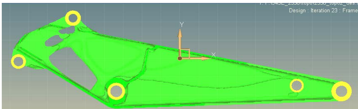
Figure 2. Topological optimization of arm 图 2. 斗杆整体拓扑优化
