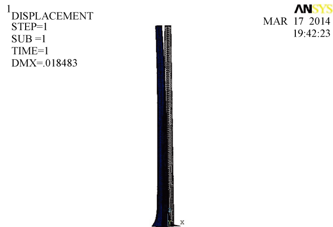
Figure 2. Tower deformation under the influence of surface tensile deformation
