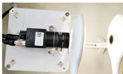
Figure 2. Positional relationship between camera lens and light source 图2. 相机镜头与光源的位置关系
