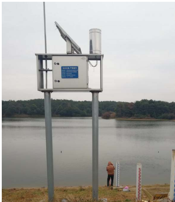
Figure 7. Construction drawing of bubble reservoir hydrological forecasting station (Xianqian Reservoir in Gao'an)
