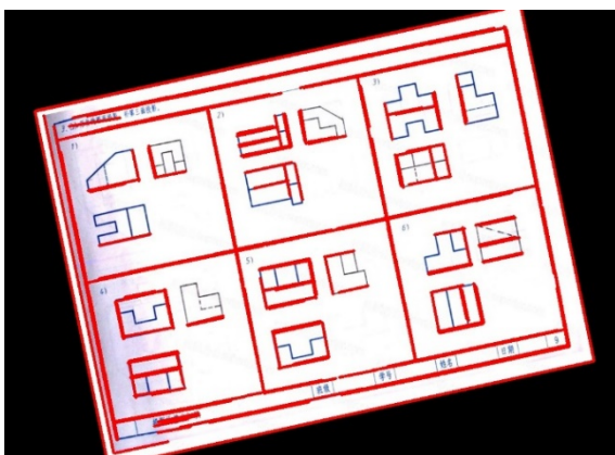
Figure 5. The straight line after Hough transform 图 5. Hough 变换的直线
