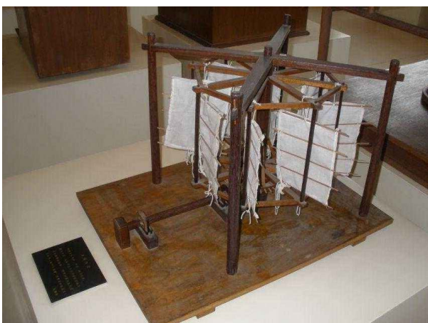
Figure 4. Vertical windmills in the Song Dynasty 图 4. 宋代立式风车
