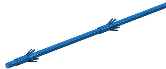
Figure 3. Combination of round barb and anchor 图 3. 圆形倒刺与锚杆组合
