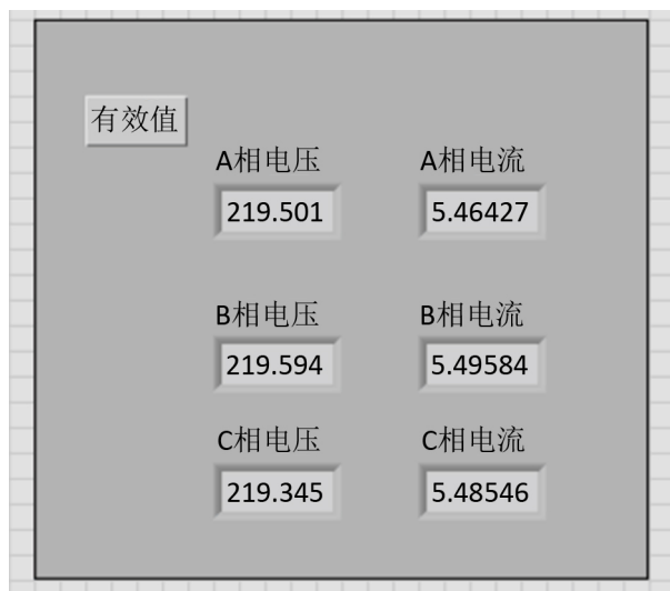
Figure 5. Three-phase voltage and current RMS front panel 图 5. 三相电压电流有效值前面板
