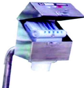
Figure 3. The sketch of the traditional of mud pit volume sensor 图 3. 传统池体积传感器示意图
