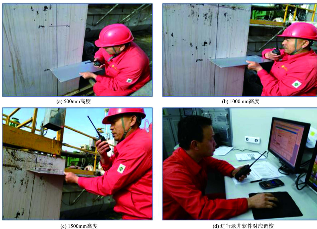
Figure 12. The method for testing multi-point calibration of sensors
