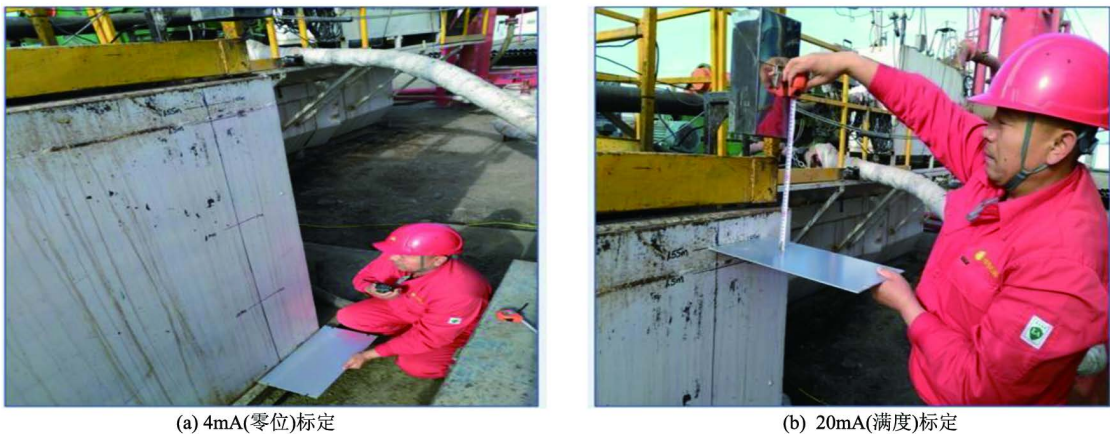
Figure 1. The calibration of zero and full level of sensor 图 1. 传感器零位、满度标定
