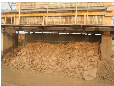
Figure 2. The mud filtering with filter press 图 2. 压滤机压滤泥浆
