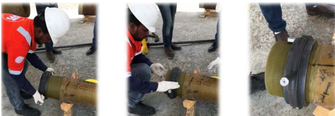
Figure 3. Measuring external thread with ring gauge 图 3. 环规测量外螺纹
