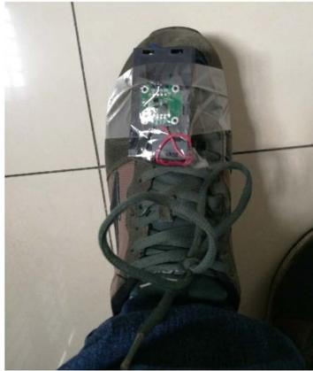
Figure 6. MPU9250 physical drawing
