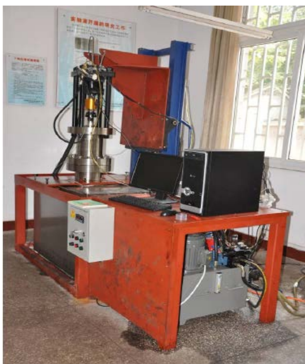
Figure 2. Triaxial stress thermal-hydro-mechanical coal containing gas permeameter
