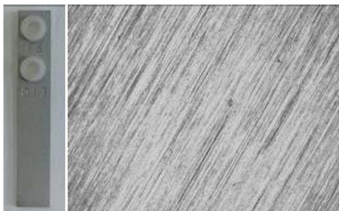
Figure 1. The surface morphology of N80 on no corrosion coupon 图 1. 未腐蚀 N80 钢挂片表面形貌
