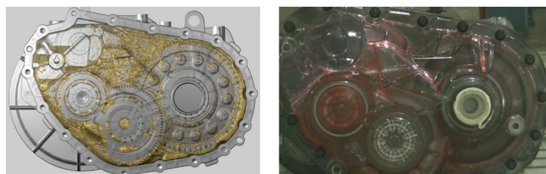
Figure 19. Comparison of simulation and test results after optimization; Left side view of oil distribution in 16.7° right tilt condition
