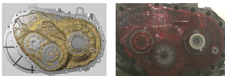
Figure 15. Comparison of simulation and test results after optimization; Left side view of oil distribution in horizontal reverse condition
