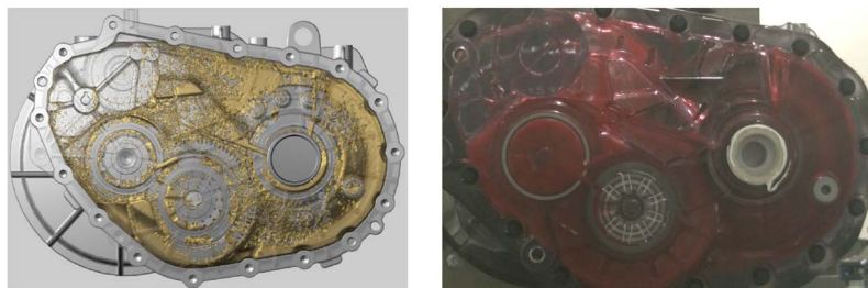
Figure 14. Comparison of simulation and test results after optimization; Left side view of oil distribution in horizontal forward condition
