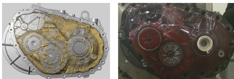
Figure 16. Comparison of simulation and test results after optimization; Left side view of oil distribution in uphill 5.7^\circ condition
