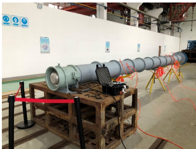
Figure 6. Field drawing of fan performance test 图 6. 风机性能测试现场图
