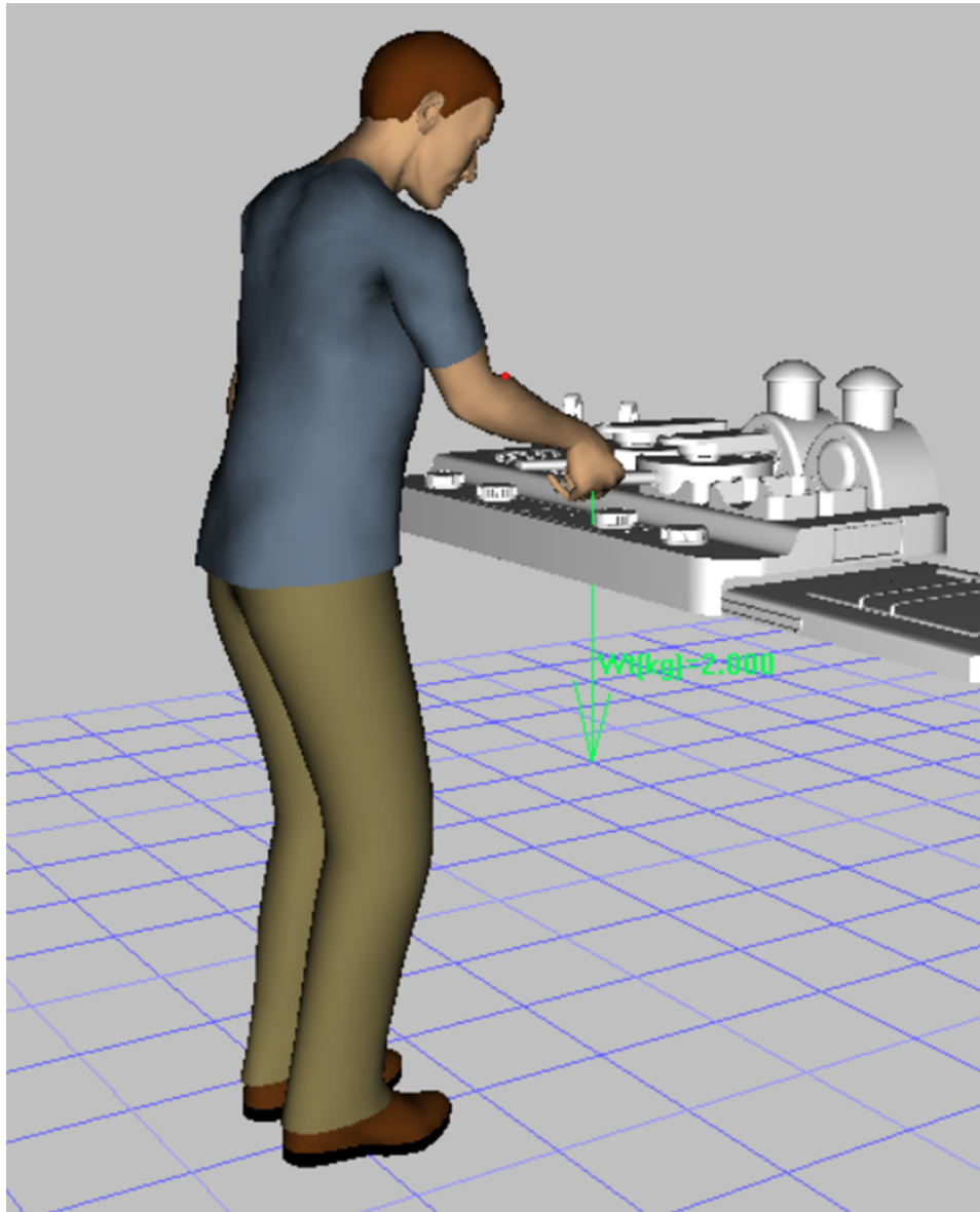
Figure 8. Apply wok weight to the hand joints 图 8. 为手部关节施加炒菜锅重量
