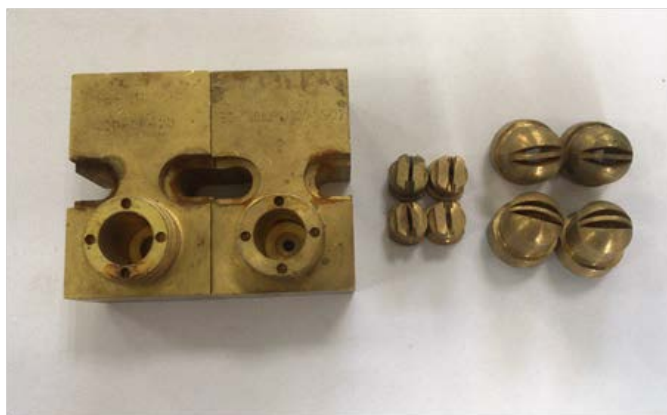
Figure 6. Base and test nozzle 图 6. 喷嘴底座和测试喷嘴
