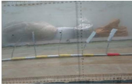
Figure 8. The test of longitudinally arranged plants 图 8. 植物沿程纵向排列模型试验
