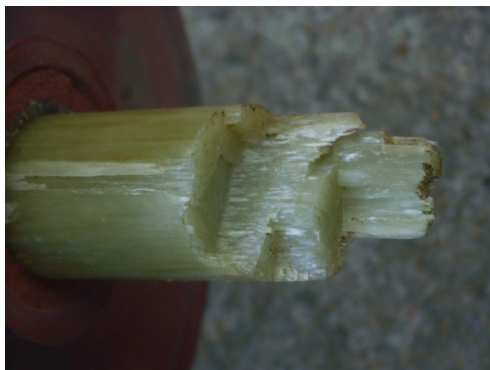
Figure 5. Brittle fracture of mandrel
