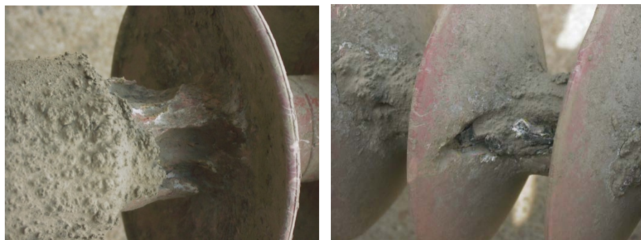
Figure 6. Composite insulators running six and a half years
