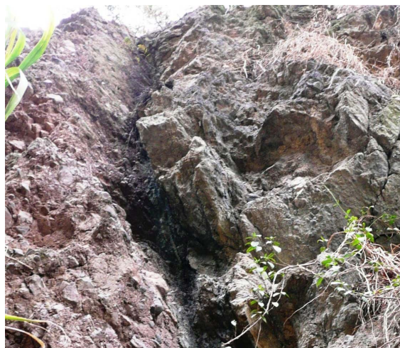
Figure 11. The grey black gouge on fracture surface of the northwest-striking fault 图 11. 北西向断裂下界面处的灰黑色断层泥
