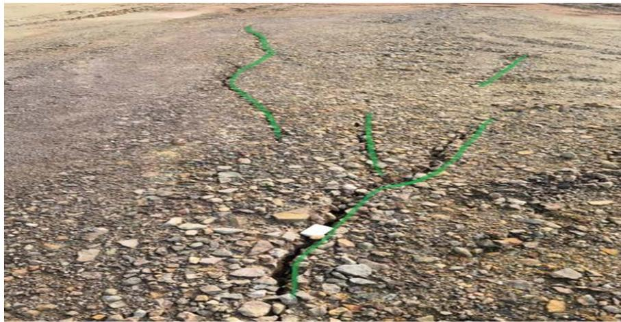
Figure 4. Ground fissures developed on the west side of Nanshan mine stope
