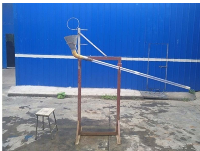
Figure 7. Testing device of inclined tube: 1—charging hopper; 2—fixed ring; 3—bracket; 4—sliding device; 5—fixed device; 6—conveying tube
