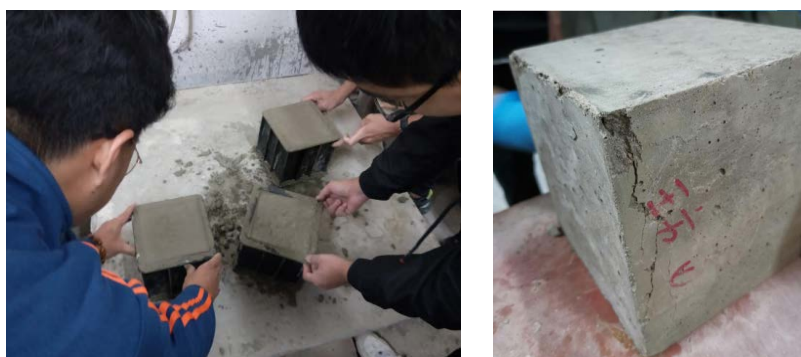
Figure 1. Students make a cube and measure the strength
