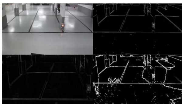
Figure 5. Comparison of canny, Laplacian and Sobel 图 5. Canny、Laplacian、Sobel 边缘检测效果对比图
