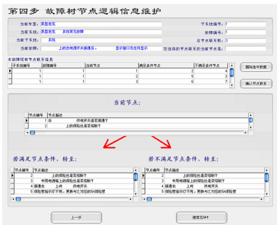
Figure 4. Logic information maintenance interface of fault tree node 图 4. 故障树节点逻辑信息维护界面
