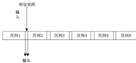
Figure 4. Edge overlap division method 图 4. 边缘重叠划分方式
