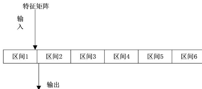
Figure 3. Uniform non-overlapping division method 图 3. 均匀无重叠划分方式
