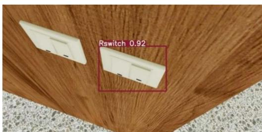
Figure 14. Detection and identification results of the switch
