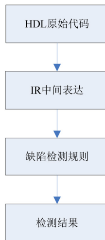
Figure 1. Flow chart of semantic defect auto detection 图 1. 语义缺陷自动检测流程图
