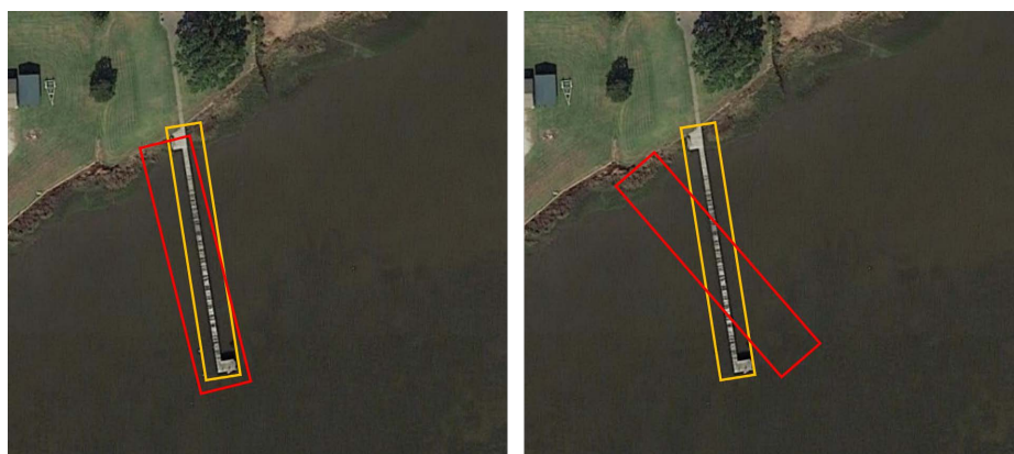
Figure 4. Effect of angular offset on objects with high aspect ratio 图 4. 角度偏移对高长宽比物体的影响
