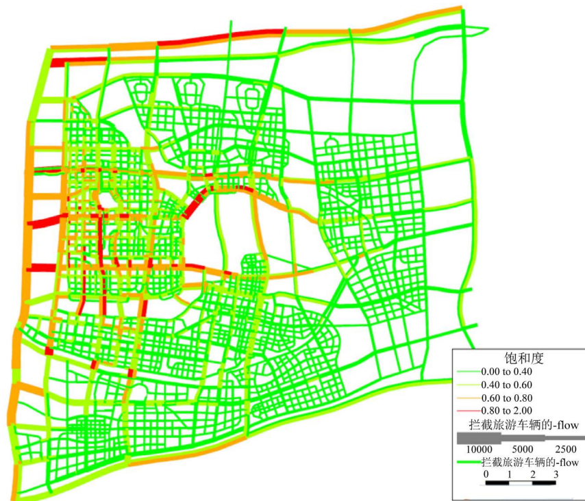
Figure 10. Saturation of road in Zhongmu with traffic management on tourist peak day 图 10. 旅游高峰日有交通管理措施的中牟中心城区路网饱和度
