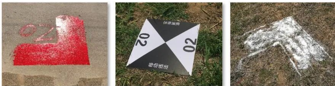
Figure 1. Types of image control points
