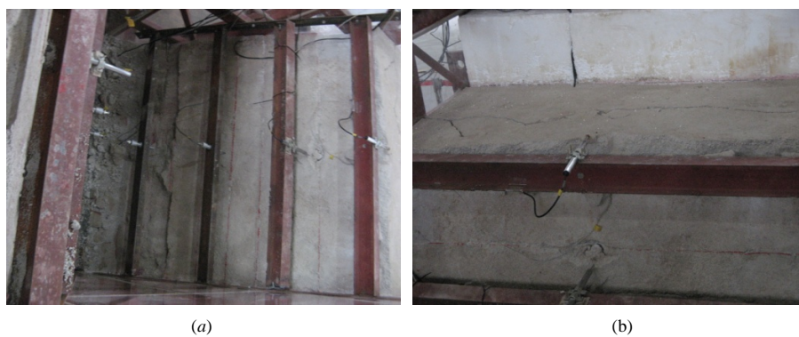
Figure 4. Cracks in model mudstone slope (a) toe of slope (b) crest of slope 图 4. 均质泥岩边坡裂纹分布 (a) 均质泥岩边坡底部裂纹 (b) 均质泥岩边坡顶部裂纹
