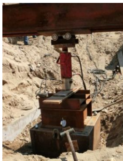
Figure 4. The vertical pressurization equipment 图 4. 垂直加压设备
