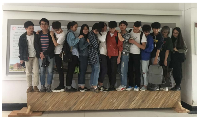
Figure 8. Loading test of short bamboo strips nailed web 图 8. 站人荷载试验
