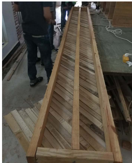
Figure 6. Skeleton of joist with short bamboo strips nailed web 图 6. 短竹片钉接腹板楼面搁栅的木骨架
