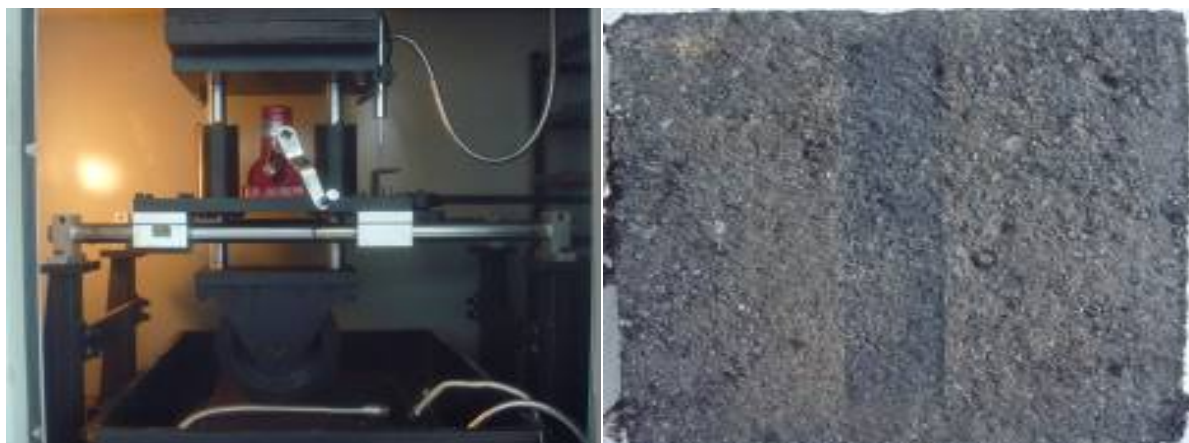
Figure 2. Rutting test equipment and test specimens
