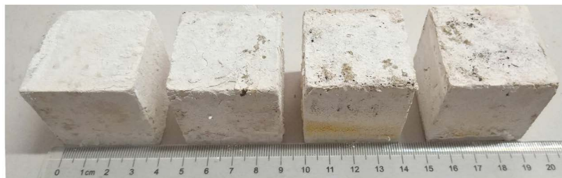
Figure 3. Samples with different raw material mix ratios (A1, A2, A3, A4 in turn) 图 3. 不同原材料配合比样品(依次为 A1、A2、A3、A4)
