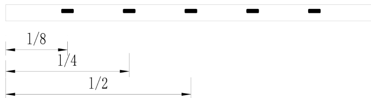
Figure 9. Carbon plate strain gauge adhesion 图 9. 碳板应变片粘贴
