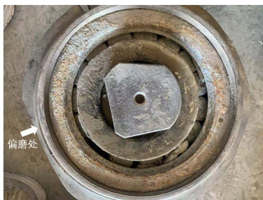
Figure 2. Knife ring eccentric grinding 图 2. 刀圈偏磨
