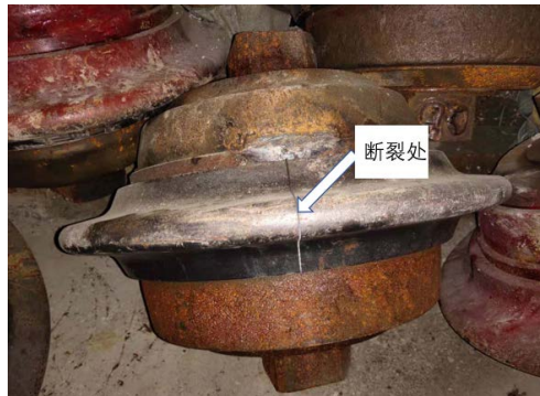
Figure 3. Knife ring break 图 3. 刀圈断裂
