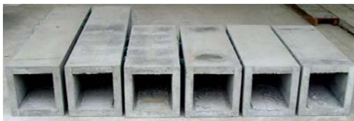
Figure 1. Prefabricated RC shell formed by core pulling 图 1. 抽芯成型的预制 RC 外壳
