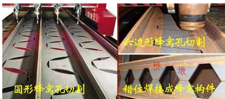
Figure 1. The manufacturing process of castellated beams
