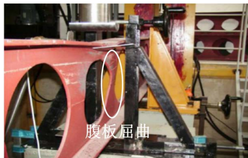
Figure 3. Web post buckling of castellated beams [9]
