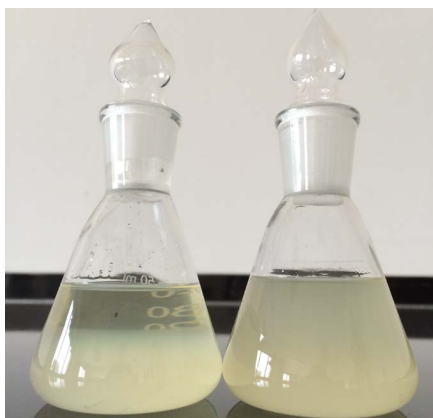
Figure 3. Dispersion of silicon dioxide in organic solvent before and after modification
