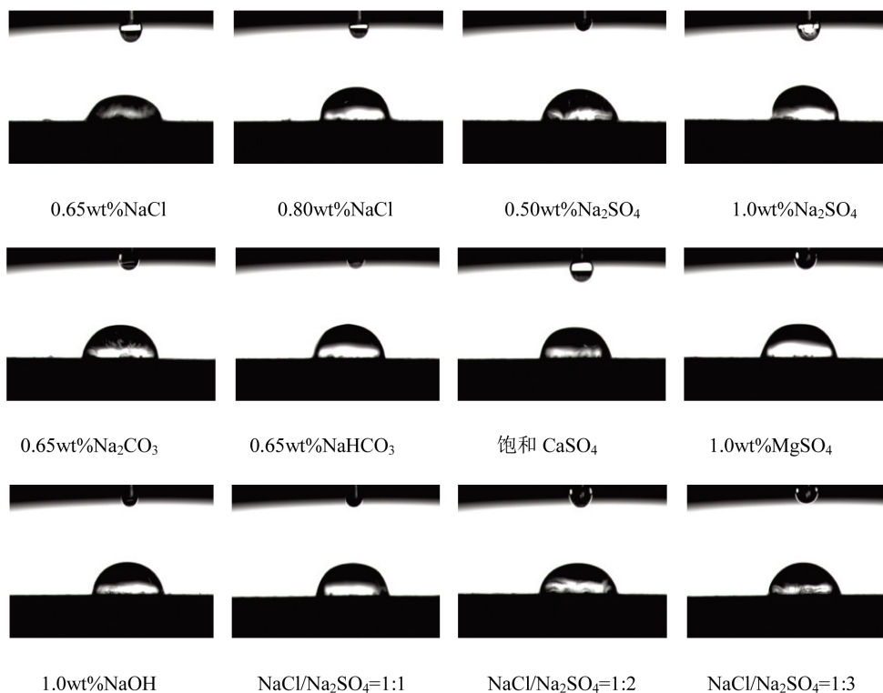
Figure 4. Contact angle test chart of salt water and coal 图 4. 盐水与煤的接触角测试图
