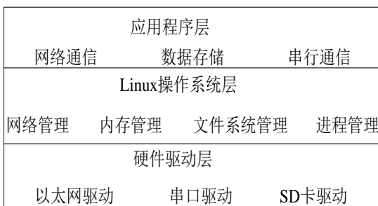
Figure 4. The level architecture of main control
