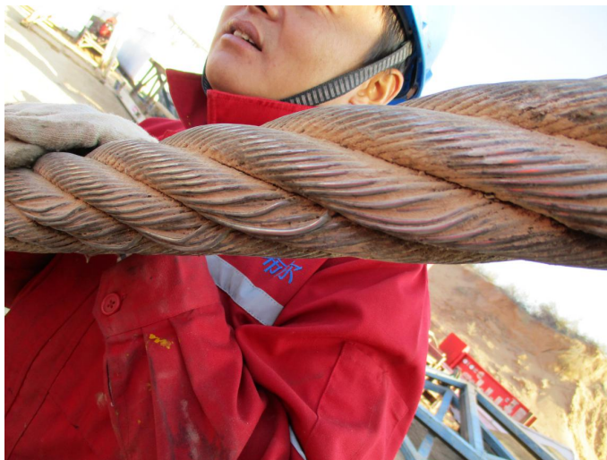
Figure 6. Photograph of verifying for hoisting wire of specification 6*37-IWSC-48
