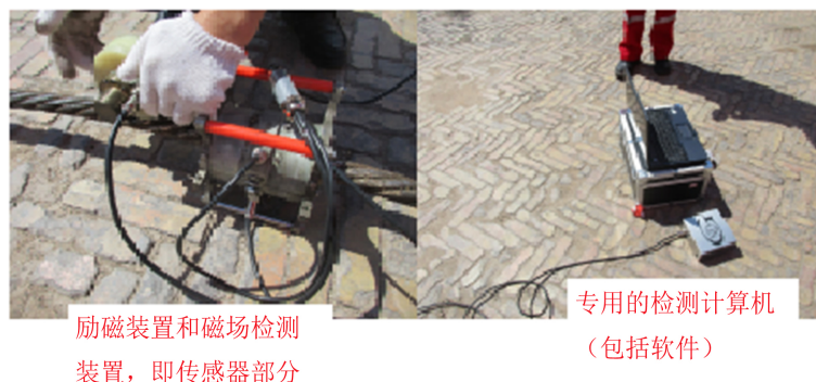
Figure 2. Components of detection instrument for hoisting wire rope
