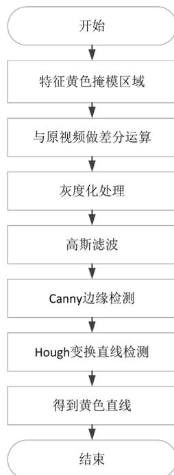
Figure 14. Process of detecting yellow line module based on Hough transform
