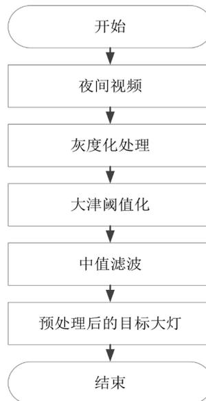
Figure 8. Pretreatment process of nighttime headlamp target
