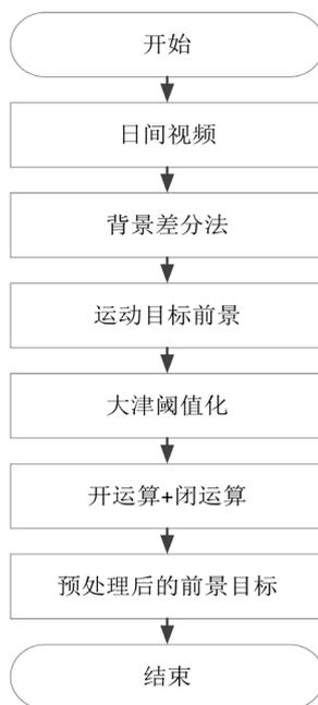
Figure 3. Foreground pretreatment process of moving vehicles
