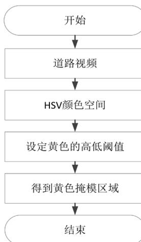
Figure 13. Process of obtaining yellow region based on HSV color space
