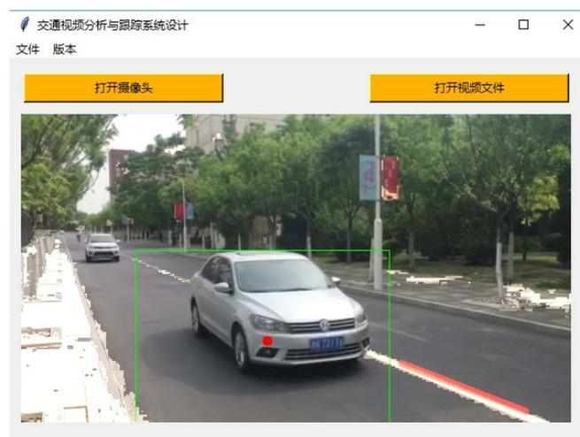
Figure 18. Example of violation detection of traffic line
