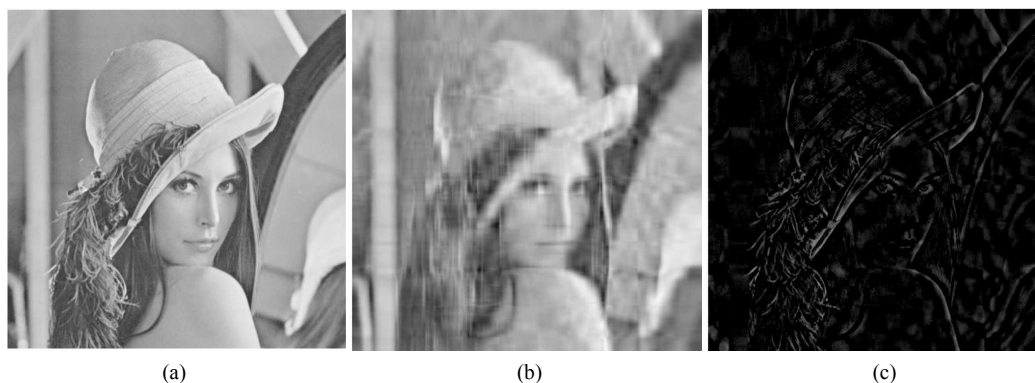
Figure 2. (a) Standard Lena images; (b) Lena image superimposed on the top 15 singular value weighted maps; (c) Remove the Lena image after the top 15 singular value weighted mapping bases are superimposed
