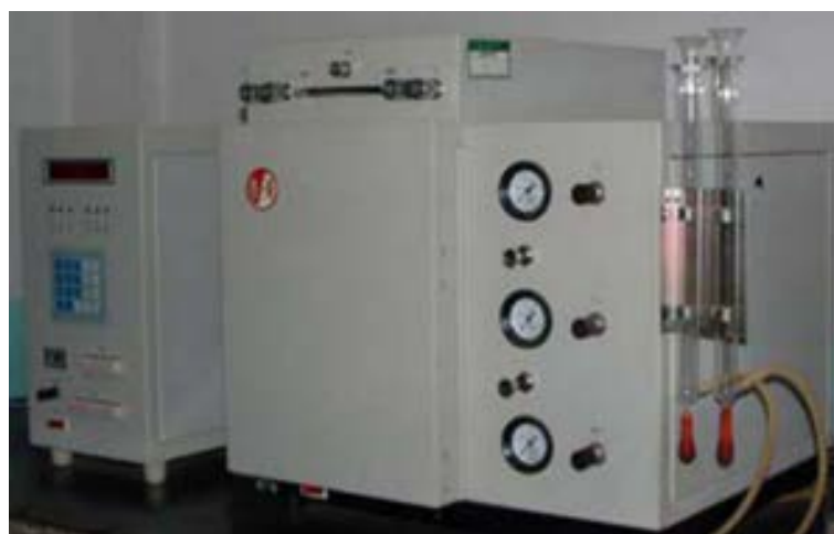
Figure 1. Model ZRJ-1 oxygen adsorption detection instrument with flow chromatograph
