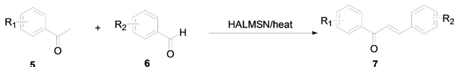
Figure 3. Synthesis of chalcone derivatives using HALMSN (Si/Al = 18.9) as catalyst
