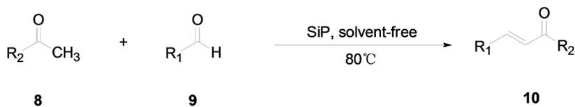
Figure 4. Catalytic synthesis of chalcone derivatives by the coupling of silica and piperidine
