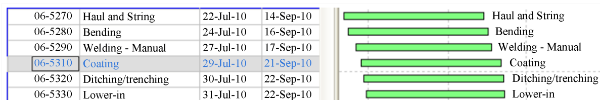
Figure 1. Typical Gantt chart of pipeline project
